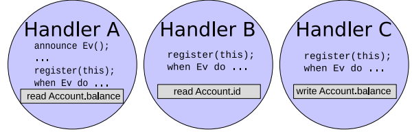
Figure 4. Assume there are three handlers for the event type Ev in the program. At this point, none have registered yet. Handler A will register first, then handler B . Finally handler C will register last. The effect set of a handler is put inside the grey rectangle.
