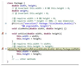
Figure 8. The crosscutting contract structure in the Package class using AspectJML/AJDT [22].
